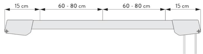
The fixing distances above are meant as a guide only, they may vary depending on the width of track and curtain weight.
