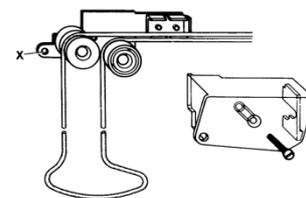
Unscrew the nylon cover. Drill a hole in the wall directly behind 'X', insert screw through hole and spacer and screw firmly into position. Then replace the nylon cover.
