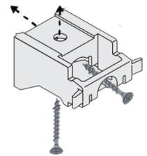
Firmly screw the brackets to wall or ceiling.
