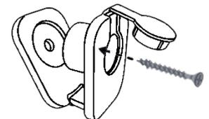
To fit the retainer, mark the position on the wall and then drill a hole. Make sure the retainer is open and place the cord round the centre part.
