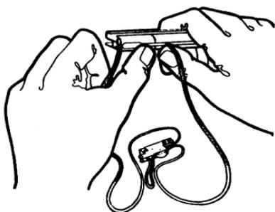
5. Pull cords through into glider channel and clear of cutting point.
