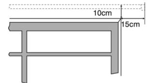
The track is adjusted in length by sliding the inner track into or out of the outer track.
