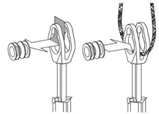
Place the cord inside the pulley and replace the barrel ensuring it clicks into place.
