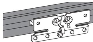
Take up the slack of the cord and tie a knot behind the Master Slide arm.
