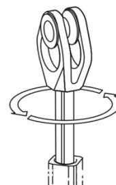
If the cord becomes twisted, simply rotate the head of the pulley to untwist it
